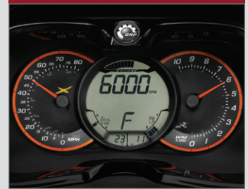
X-Gauge with boost indicator
