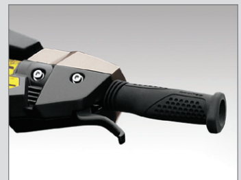
iBR (Intelligent Brake & Reverse) lever
