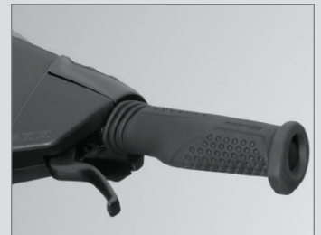
iBR (Intelligent Brake & Reverse) brake lever
